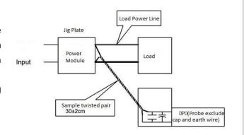
2. Schematic diagram of output ripple noise test:
